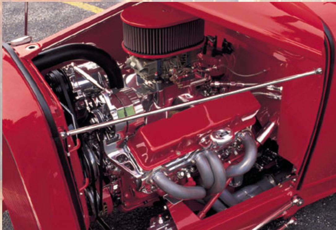
A 383-inch solid lifter cam and Brodix-head-equipped smallblock powers Jack Troup's '32 Ford Coupe.
