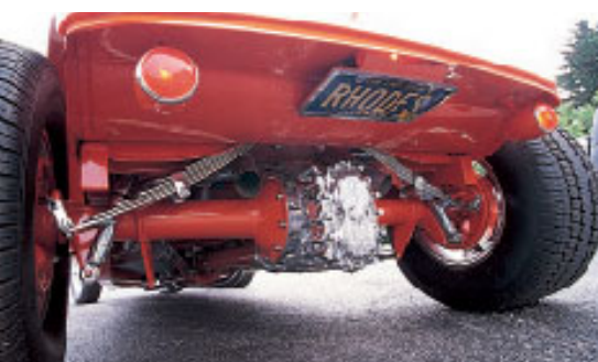
It's hard to beat a Halibrand quickchange framed by the graceful arc of a Model A rear spring. We like the smaller V-8 quickchange rear ends in Model A's and Deuces, but the larger Champ quickchange looks equally at home in a '33-'34 Ford
