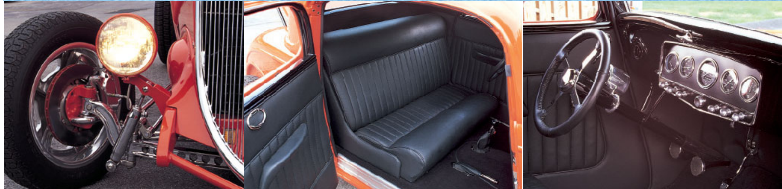
Rhodes' coupe screams traditional hot rod in stance, silhouette, detailing and componentry. Wheels are 16 x 10 ET 11s in the rear and spindle-mount Halibrands in the front. Black pleated upholstery is nicely accentuated by a Bell 4-spoke wheel and a Stewart Warner equipped Auburn gauge panel. Note that the early Ford side bells bolt to the Champ quickchange with polished aluminum step-down adapters.
